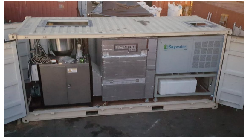
Watertainer- Biomass powered atmospheric water generator with biochar and heat
